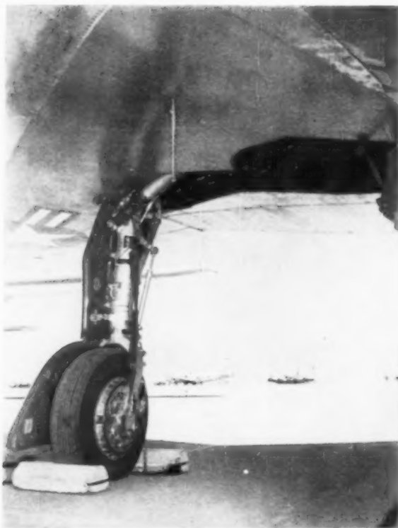
MAIN GEAR of McDonnell F-101 reflects Naval design requirements in position of lines on rear face of leg where crash barriers would not rip them off. But 150-kt. landing speed can rip tire treads; the debris wipes off lines on the rear of the leg. Lines are now being relocated to the front.
